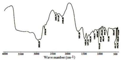
**Fig. 5.** IR spectrum of polyvinylpyrrolidone/organo-bentonite nanocomposite
