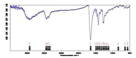
Fig. 4. IR spectrum of the starting polyvinylpyrrolidone
