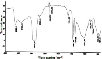
Fig. 2. IR spectrum of starting montmorillonite
