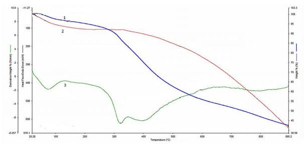
Fig. 3. Thermogram of the Zn (II) complex. 1 - TG, 2 - DTG, 3 - DTA.
