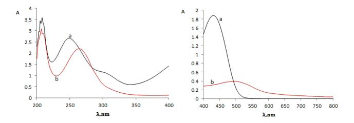
Fig. 1. Electronic banding spectra of: a) polyimine, b) Cu (II) complex with polyimine
