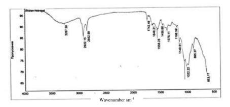
Fig. 4. IR spectrum of cross-linked chitosan.
