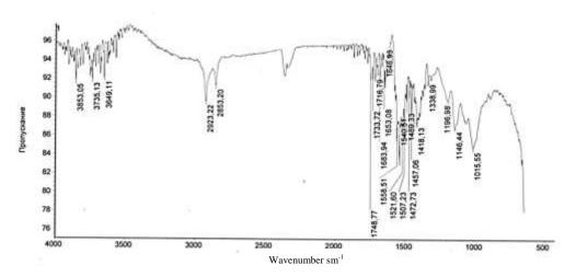
Fig. 6. IR spectrum of levofloxacin complex with chitosan-based hydrogel.
