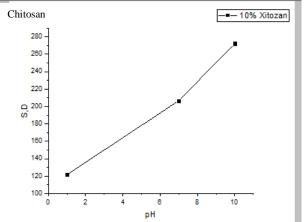
Fig. 1. Graph of the swelling degree of chitosan-based hydrogel depending on the pH of the medium.
