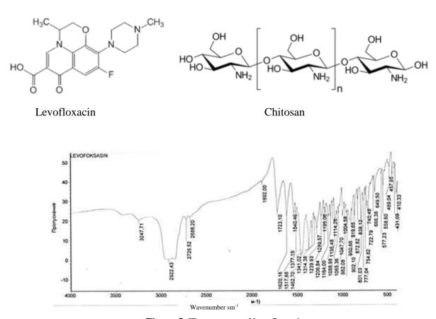
Figure 5. IR spectrum of levofloxacin.
