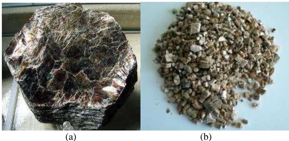
Fig. 1. View of vermiculite from Tebinbulok mine in natural (a) and porous (b) state
